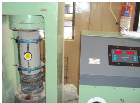
Figure 4 Test setup for Young's Modulus of concrete.
