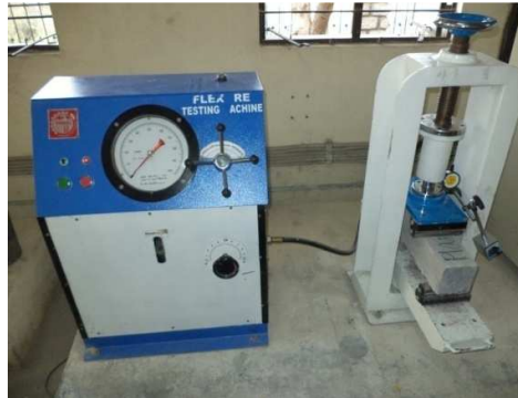
Figure 5 Test setup for flexural testing.
